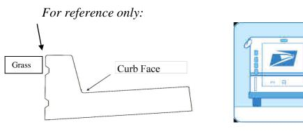
**Note:** To maintain uniformity and to determine the placement of the mailbox; during installation, a plumb bob should be hung from the front edge or hinge of the mailbox door, to the top of the curb where it meets the grass. This is the position where the mailbox should be installed.
